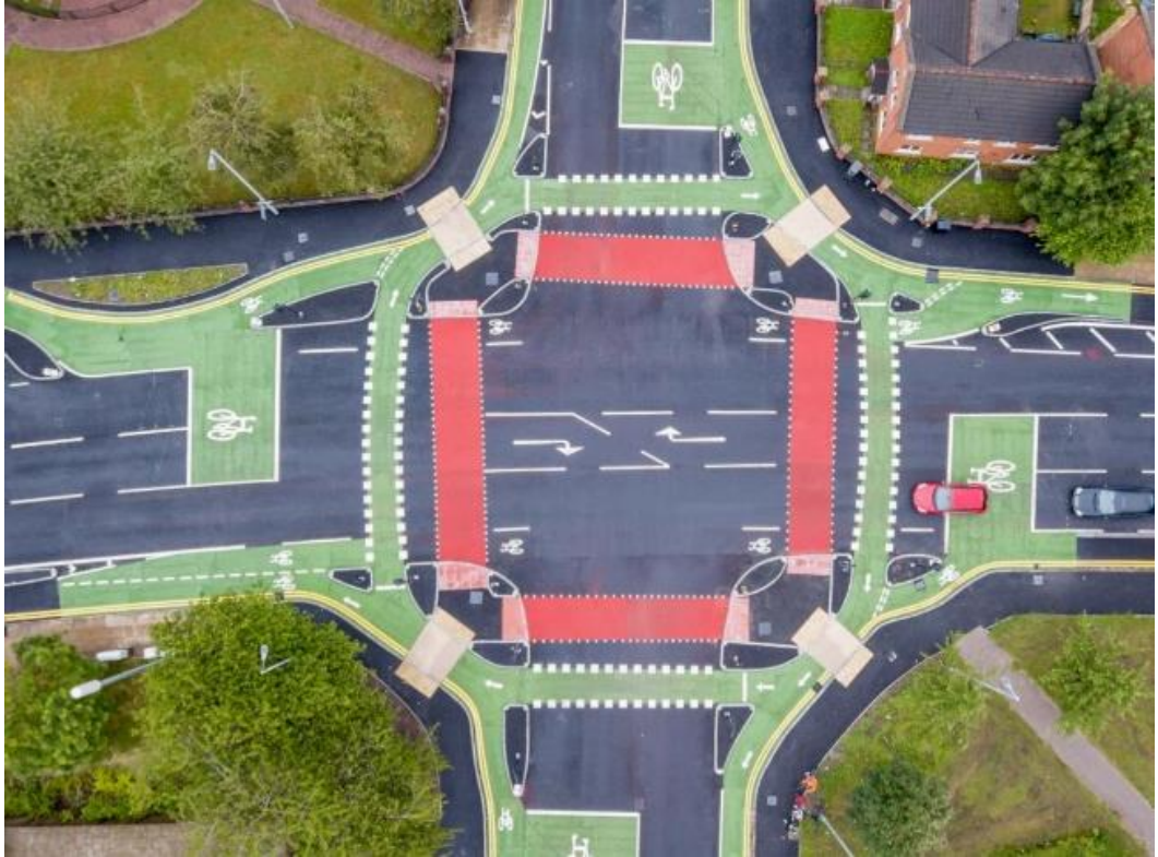
Figure 12: Aerial view of the first completed CYCLOPS junction in the UK: Hulme, Manchester
