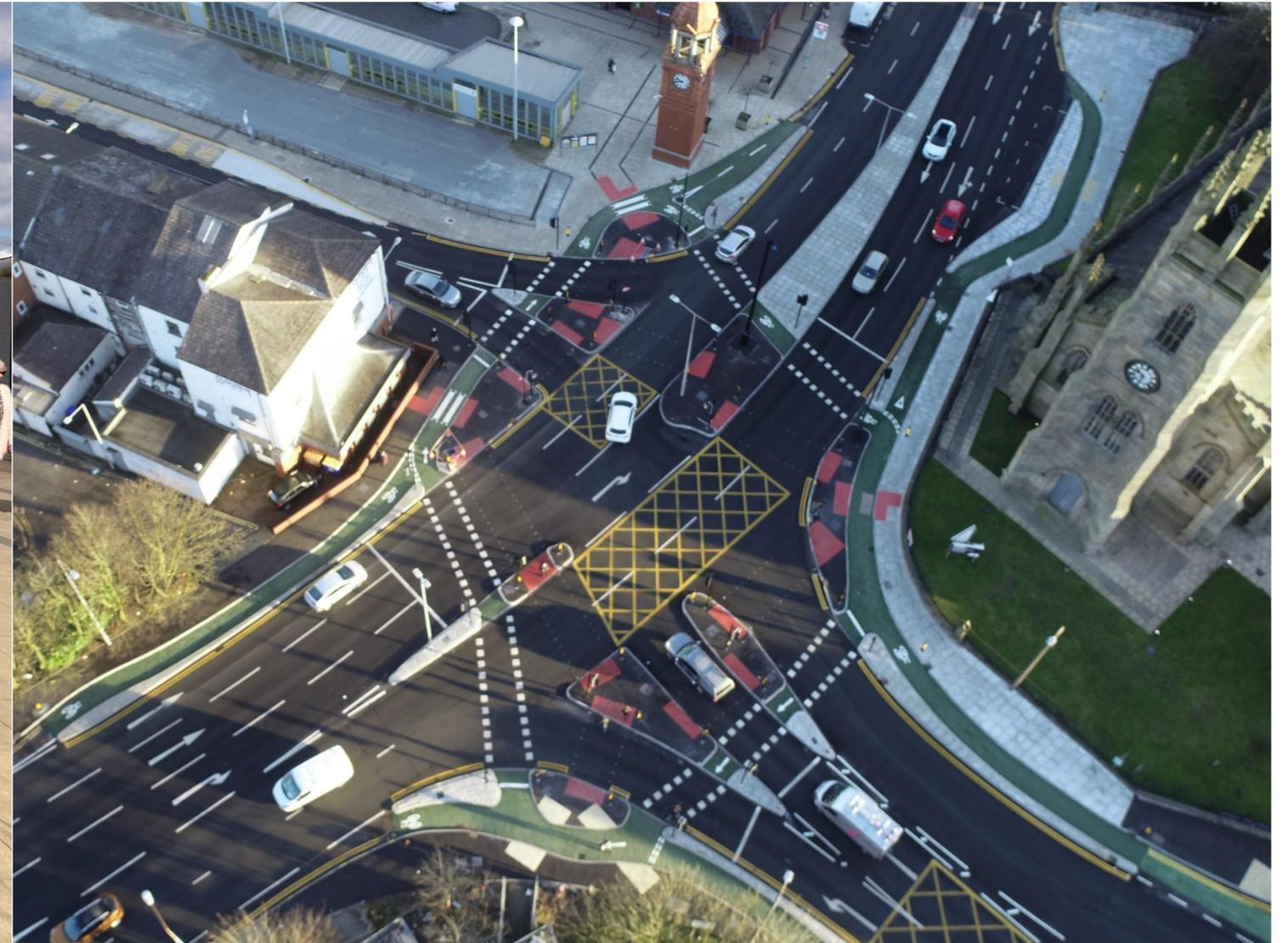
**Cyclops junction give walking, wheeling and cycling access to Bolton Bus Interchange and Railway Station**
